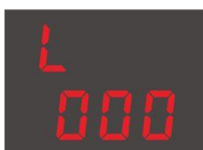
Real time display of leakage current
