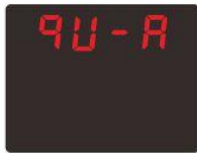
A-phase missing phase
